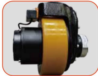
Adopt 1.3KW AC horizontal drive and equipped with 250x80 drive wheel ensure stronger carrying capacity; high power and accelerated stability, low maintenance cost as no need to replace the carbon brush; good ramp starting performance. Both sides are equipped with spring regulating structure stability castors ensure better wear resistance and stability.
