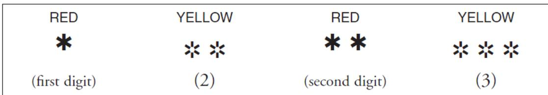
The numerical codes used by the yellow LED are listed in the troubleshooting table, which also lists possible fault causes and describes the conditions that set and clear each fault.
