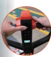
The function of driving with tiller in the **vertical position** helps with work in confined areas, especially in elevators and lorries without sacrificing of safety.
