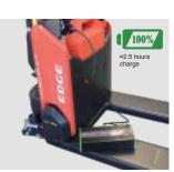
Socket on battery case for easy battery charging without necessity to take the battery out Fast and opportunity charging during brakes in operations increases working time.
