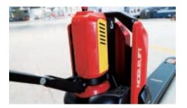
Convenient and fast access to any component of the truck, no elements are located in areas difficult to reach. No Special tools are required.
