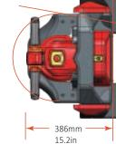
Strong steel apron protects the operator's feet during work and secures the truck's components from collisions with objects.
