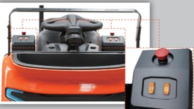
The jog button on both sides of the truck allows the operator to operate truck forward/ backward or lift the fork while walking beside. There is no need for the operator to get in and out of the truck frequently to operate it. That greatly improved the picking efficiency and operation safety by reducing the speed controlled by the jog button.
