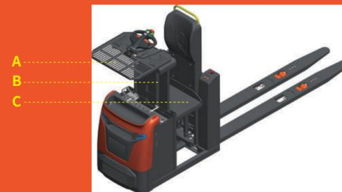
**A:** The storage platform used with the lifting operation platform allows putting or retrieving more cargo and make work more efficient.
