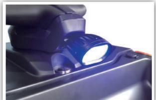
The standard blue light does not only automatically lit while the truck forwarding but also follows the handle to turn while the truck turns. It greatly improves the safety of the operation.
