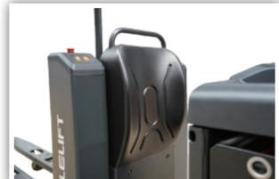
Safety flanks and non-slip surface materials on both sides of the backrest ensure the operator not to be thrown off while the truck turns at high speed. This design greatly improves the safety of driving. Meanwhile, the handle above the backrest provides a grasping point for the operator when get up or down the truck, provides superior comfort for the operator.
