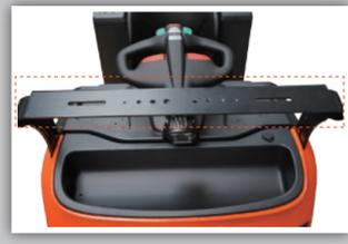
A variety of extension supports are available to meet the installation requirements of different extension equipment, such as WMS display, barcode scanner, storage tray, file plywood, etc.
