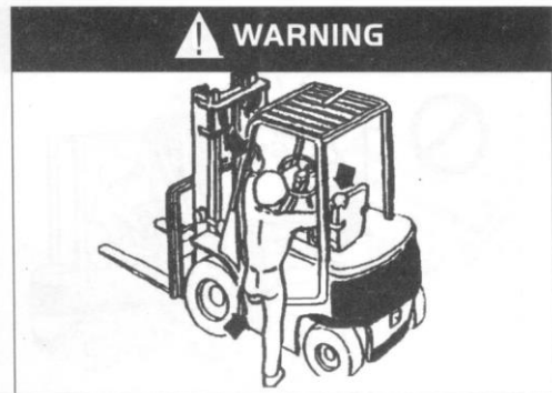
Hold the handrail during on-boarding
