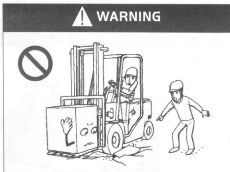
Avoid driving on soft or unprepared ground . Drive on flat and solid surface!
