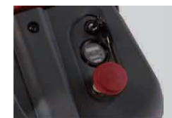
Control elements Key-switch, emergency switch and battery discharge indicator.
