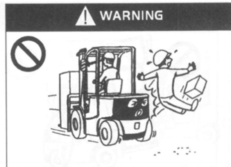
Driving Too Fast Will Result In Unstable Gravity Center And Overturning
