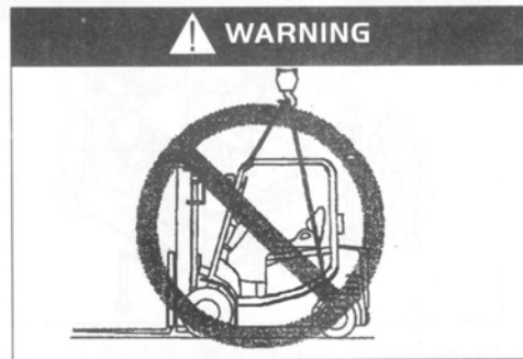
Forbidden To Hoist From Mast
