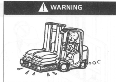
If Can Not See The Front When Turning, Please Whistle And Drive Slowly. Use Appropriate Pallet Or Sleeper When Carrying Small Object
