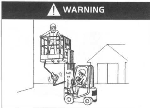
Must Use Special Equipment To Lift People Safely To Work At Height Do Not Overload
