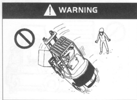
Driving Too Fast Will Result In Unstable Gravity Center And Overturning
