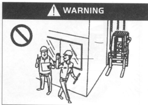
If Can Not See The Front When Turning, Please Whistle And Drive Slowly. Use Appropriate Pallet Or Sleeper When Carrying Small Object
