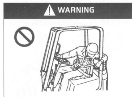
Do Not Drive On Soft Or Uncleaned Ground, Only Allowed To Run On Solid And Flat Ground .Keep Your Body Under Overhead Guard.
