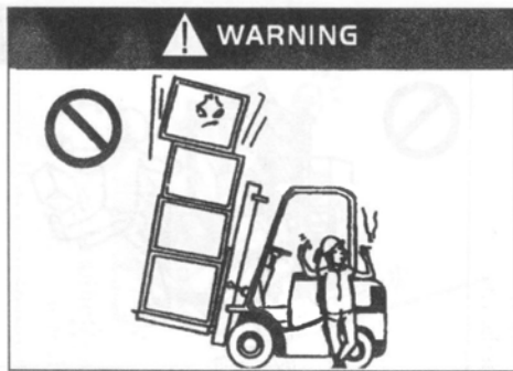
Try To Prevent Loads From Exceeding Backrest Fasten The Goods Which Is Difficult To Bind Before Loading
