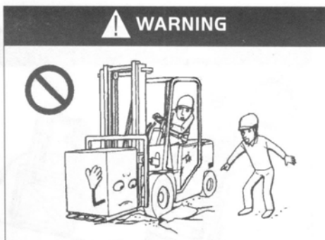
Do Not Drive On Soft Or Uncleaned Ground, Only Allowed To Run On Solid And Flat Ground .Keep Your Body Under Overhead Guard.
