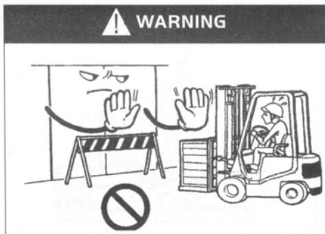
Work In Specified Area
