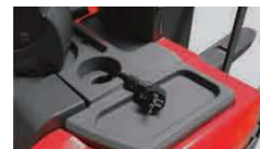
Built-in charger The built-in charger gives higher autonomy during the application.
